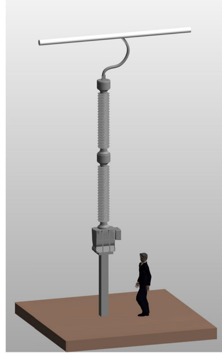
CAPACITIVE VOLTAGE TRANSFORMER (CVT)
