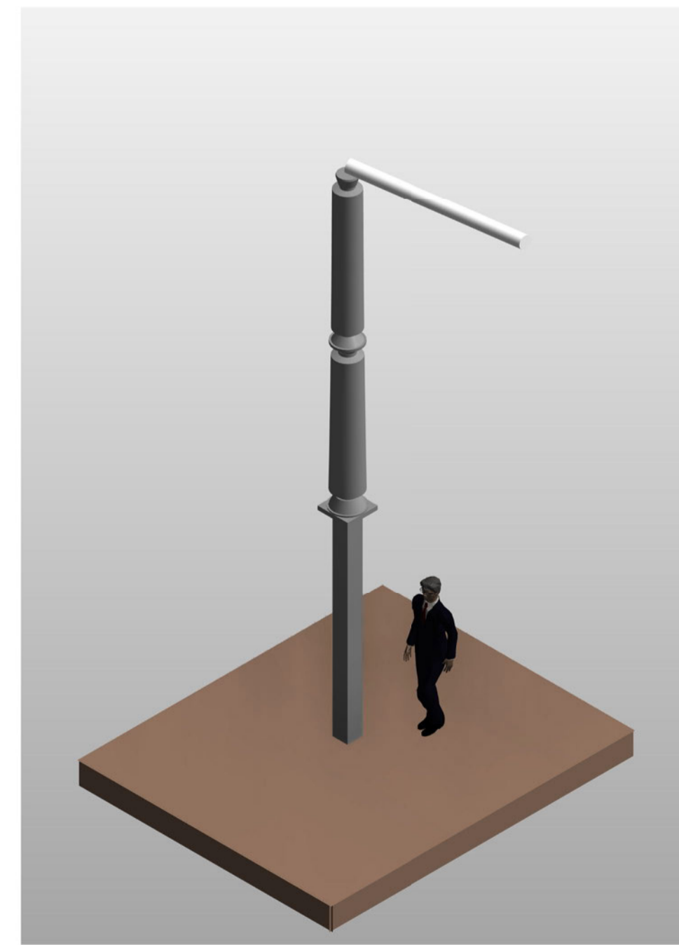
SINGLE POST INSULATOR
